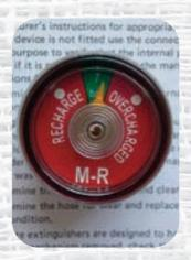
why your extinguishers should be serviced- note this faulty gauge removed yet still shows pressure OK!
