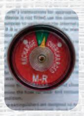
why your extinguishers should be serviced- note this faulty gauge removed yet still shows pressure OK!
